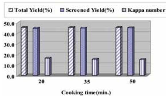
Fig. 2 Effect of cooking time on kappa number of wheat straw soda-AQ pulp
